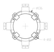
Fig.2. Bottom Fixing holes
