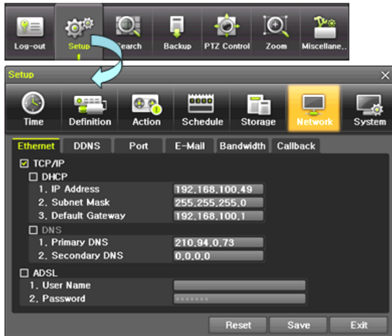
[Figure 6-46. Setup Network Window]
