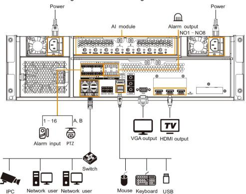
Figure 3-7 Connection diagram
