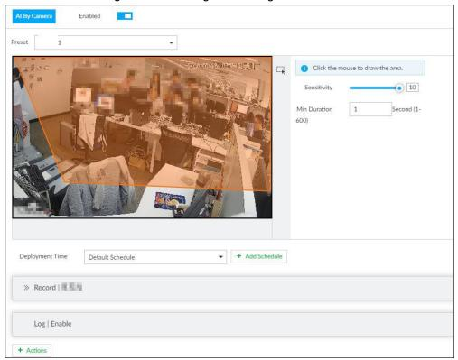
Figure 6-109 Configure smoking alarm
