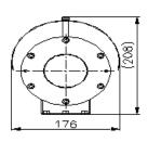
Figure 1.4.1 Dimensions of SVEX-T100 WITHOUT WIPER / SVEX-T300 WITH WIPER Explosion-proof Camera
