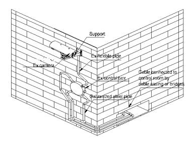
Figure 2.4.1 installation of camera
