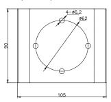
Figure 1.4.2 Distribution of installation holes of SVEX-T100 WITHOUT WIPER / SVEX-T300 WITH WIPER Explosion-proof Camera
