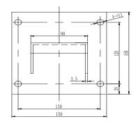
Figure 2.3.1.1 Installation of support
